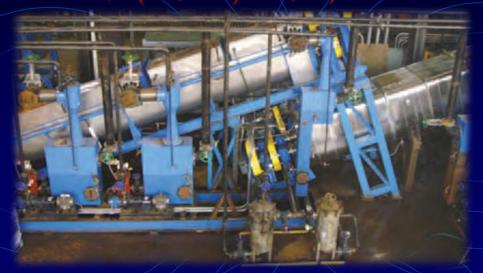
Holo-Scru® thermal dryer unit first stage and Electric-Scru thermal dryer unit second stage Such systems are excellent for delisting RCRA waste. Drums, cans, glass and plastic containers are just some of the items that carry hydrocarbon-laden materials such as paint, perfume, degreaser, oil, resins, and hair spray.
