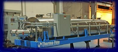
within the rotor and housing which generate process temperatures over 1000°F without the excessive volume of off-gases associated with direct-fired technologies.
