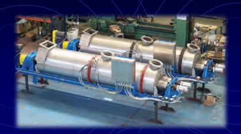
Electric-Scru® thermal desorption units is able to heat residual material up to 1,200-plus-degrees Fahrenheit, so that hydrocarbons and water vapor are condensed and recovered.
