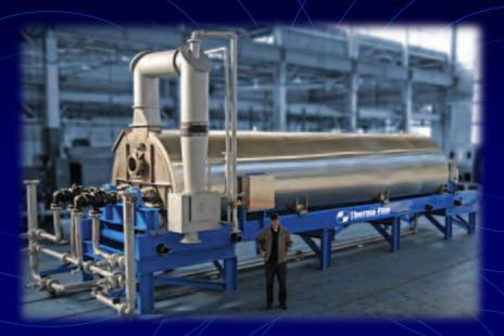
Holo-Scru® thermal desorption systems volatilize and recover 99.5% of hydrocarbons from drilling mud.
