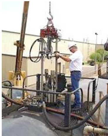
Photos 1a and 1b. Installing telescopic washing apparatus in tank car manway
