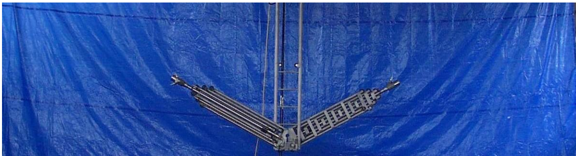
Photo 2. Unfolding telescopic apparatus
